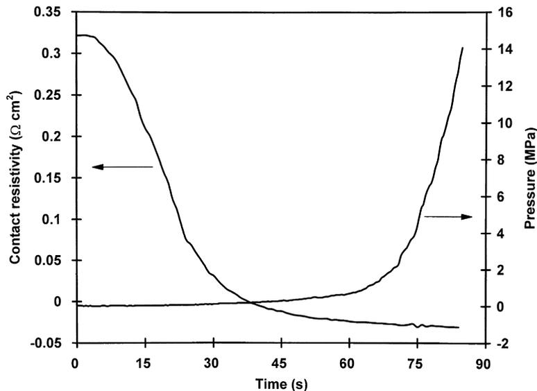
Fig. 10. Variation of apparent resistivity and of pressure with time during compressive loading of crossply laminae having no matrix.
