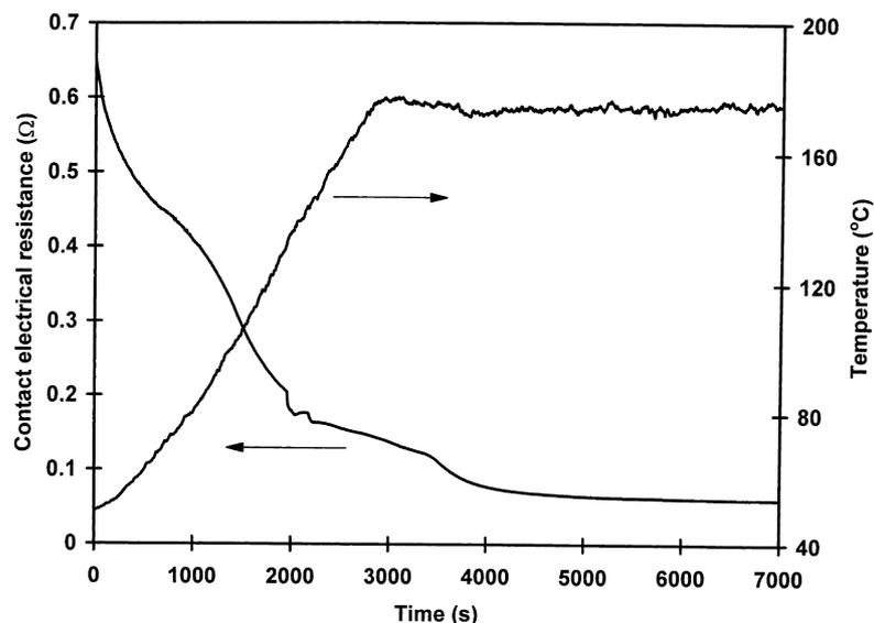
Fig. 6. Variation of apparent resistance during curing at 0.13 MPa of a two-lamina crossply sample.
