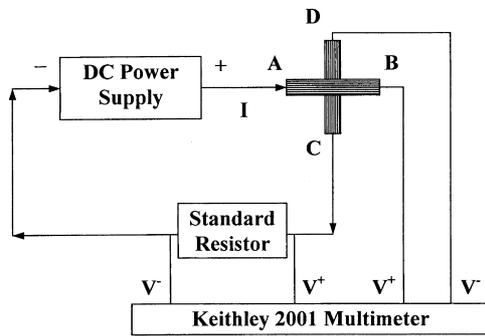
Fig. 2. Experimental set-up for obtaining current–voltage characteristics.
