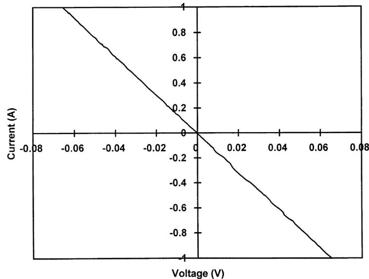
Fig. 4. A typical current–voltage characteristic for sample cured at 1.4 MPa.
