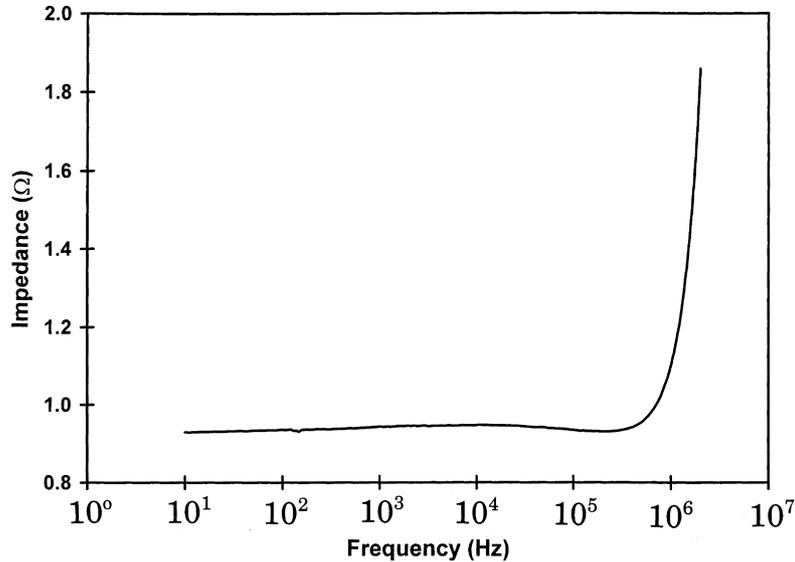
Fig. 12. Plot of apparent impedance magnitude versus frequency for carbon fiber cement–matrix composite.
