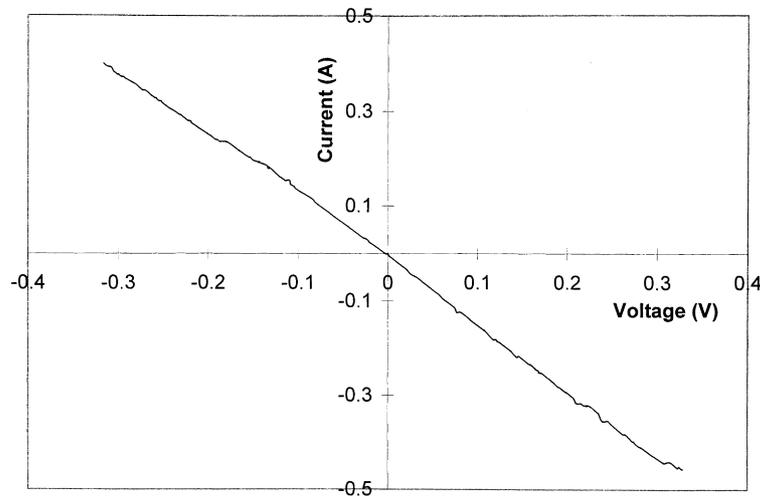
Fig. 11. A typical current–voltage characteristic for cement–matrix composite.
