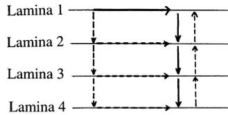
Fig. 13. Schematic of a four-lamina composite illustrating current flows resulting in zero apparent resistance. The flow indicated by solid arrows occurs because of the volume resistance within a lamina in the through-thickness direction making this flow more favorable than in the case of a two-lamina composite exhibiting apparent negative resistance. The flow indicated by upward dashed arrows is the backflow.
