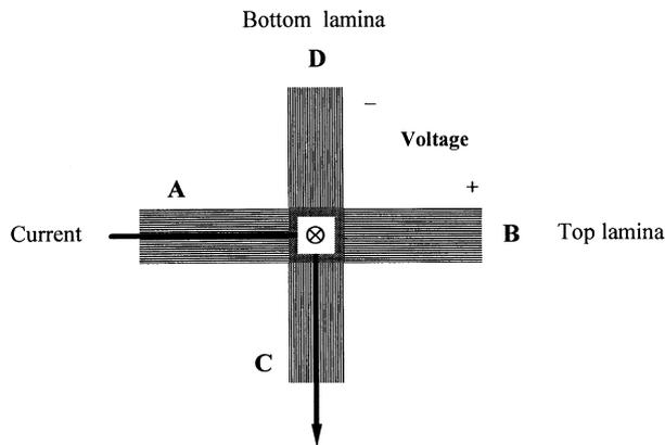
Fig. 1. Composite configuration for electrical measurement.
