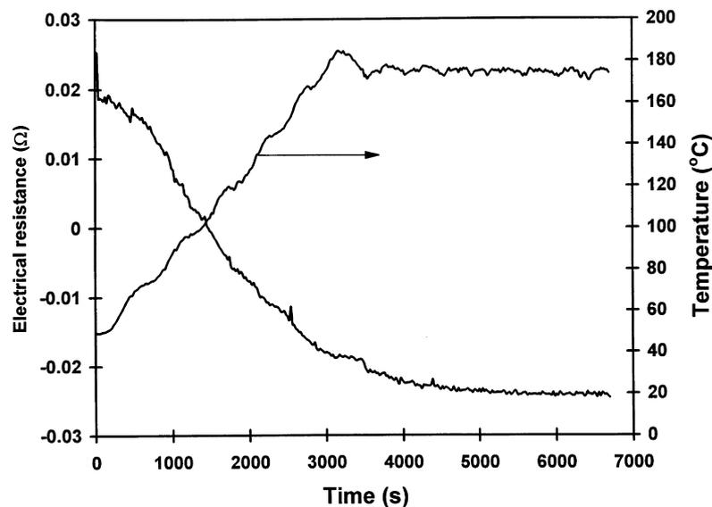
Fig. 8. Variation of apparent resistance during curing at 1.4 MPa of a four-lamina crossply sample.
