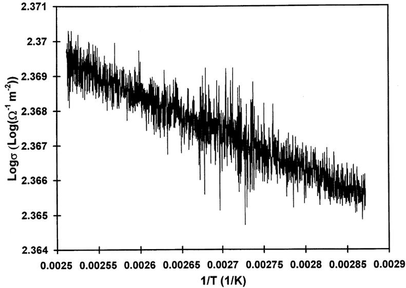
Fig. 9. Arrhenius plot of the logarithm (to the base 10) of the apparent conductivity versus the inverse absolute temperature for sample cured at 1.4 MPa during cooling.
