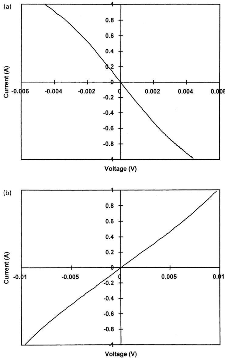
Fig. 5. Two types of current–voltage characteristics for sample cured at 0.33 MPa. (a) Negative slope. (b) Positive slope.
