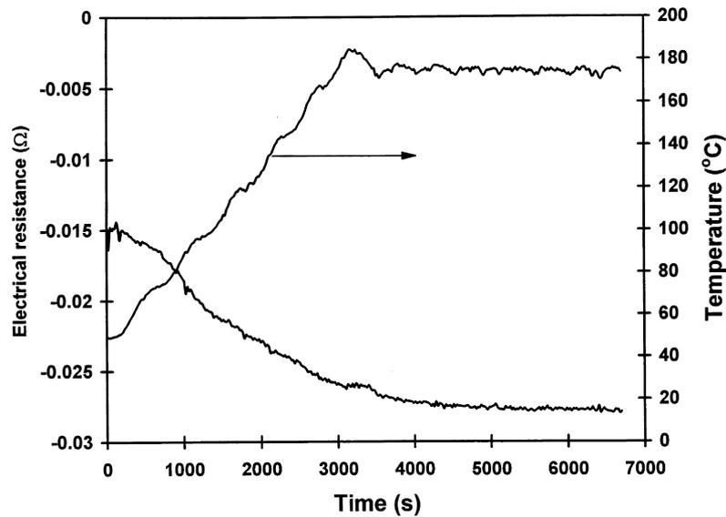
Fig. 7. Variation of apparent resistance during curing at 1.4 MPa of a two-lamina crossply sample.
